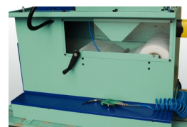
Collecting and filtering equipment for the cooling mixture complete with watersprout for cleaning
