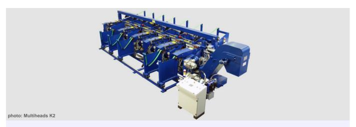
Complete system with independent heads and positioning based on length with magazine loader. Included with single chains with photocell sensor to avoid the surcharge of the tubes.
